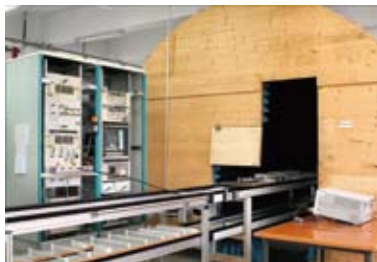
Anechoic Chamber: Excellent testing environment for antennas
